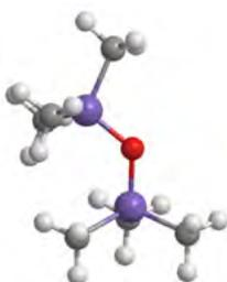
Silanes and siloxanes, the two most common types of water repellents, are both derived from the silicone molecule. Silicone is a generic name for a wide variety of polymeric chains constructed around a molecular backbone of SILICON - OXYGEN - SILICON (image at left). Despite being very closely related, silanes and siloxanes they have significant performance differences that will be explained below. But first, here are general similarities between silane and siloxane sealers:
