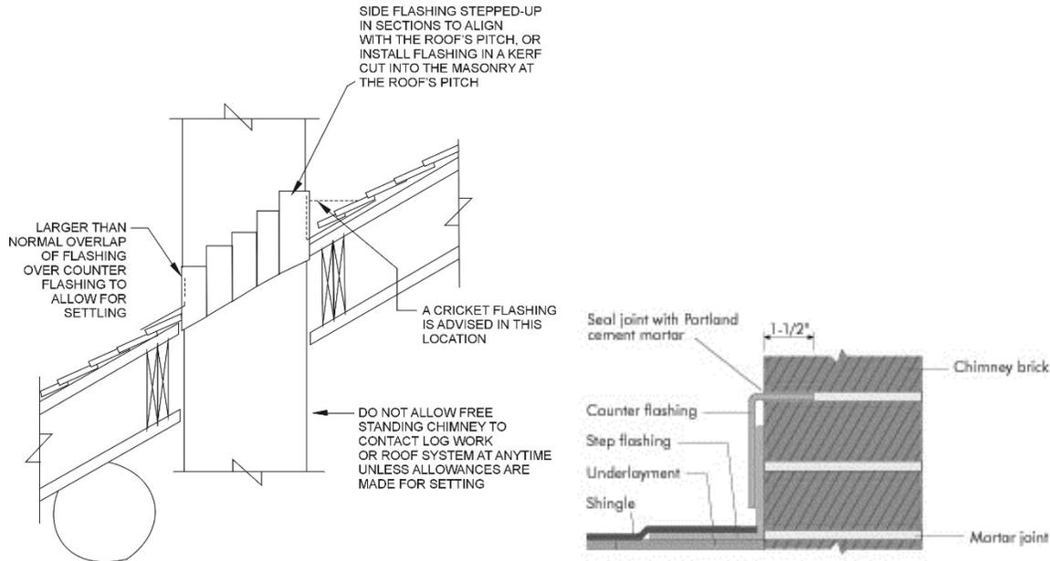
Fig. 4.3.3.4 Chimney flashing details (step-by-step) published by the APA Better Built Home program (2006).
