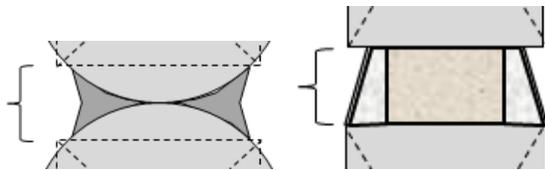
Fig. 4.1.3.2. Fully round logs may vary in relation to the log below from touching to separate like its rectangular counterpart. (Illustration courtesy of TimberLogic LLC).
