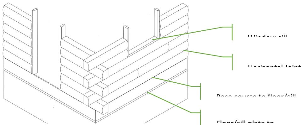
Figure 4-1 Horizontal joints in a log wall
