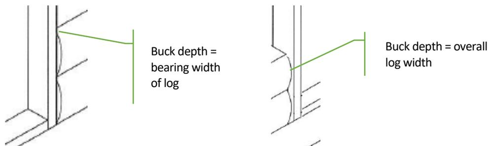
Figure 4-7 The depth of the rough buck relative to the log profile will affect the method of sealing and trim.
