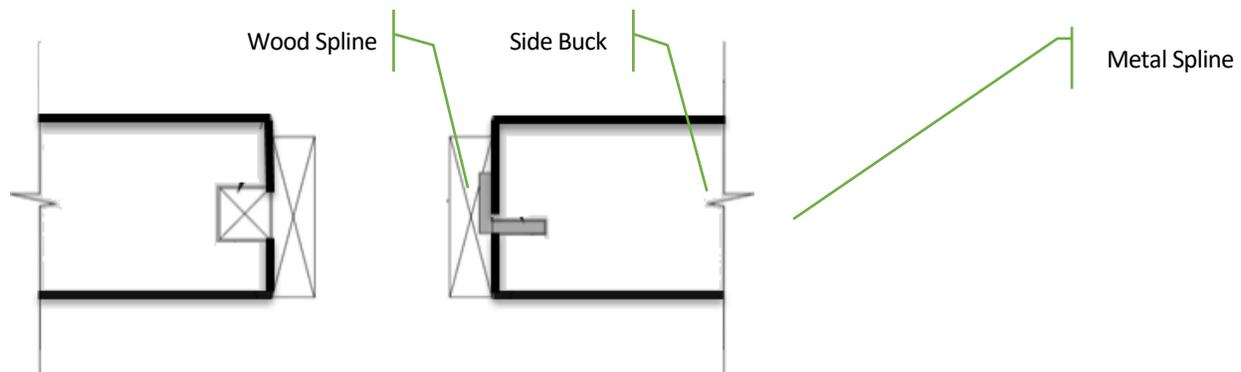
Figure 4-8 Options for connecting the log ends to the buck that offer alignment and vertical movement.
