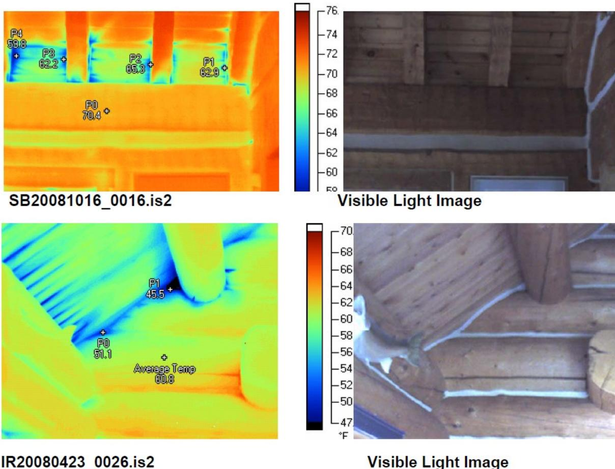
Figure 2-3 Infrared photos indicating air leakage above the log wall to the roof deck (courtesy Tracy Hansen, Stormbusters, Inc.). Top photos show leakage in the “birdblock” area above the log wall and between rafters. The bottom photos show leakage where decking bears on the log wall in a purlin roof system.
