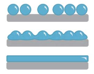
The water-based sealer drying mechanism is irreversible; that is, the dried sealer cannot be re-dissolved in water and is quite resistant to other solvents. Also, if the water and coalescing solvent do not evaporate in the proper sequence due to environmental conditions or improper application, the coalescence and drying of a water-based sealer will be flawed, leading to sealer appearance and performance problems that are difficult or sometimes impossible to fix.
