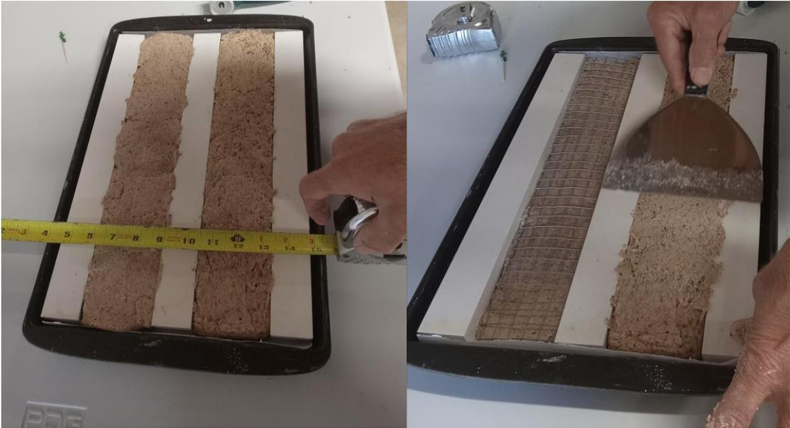
Figure 12a. Check beam widths
