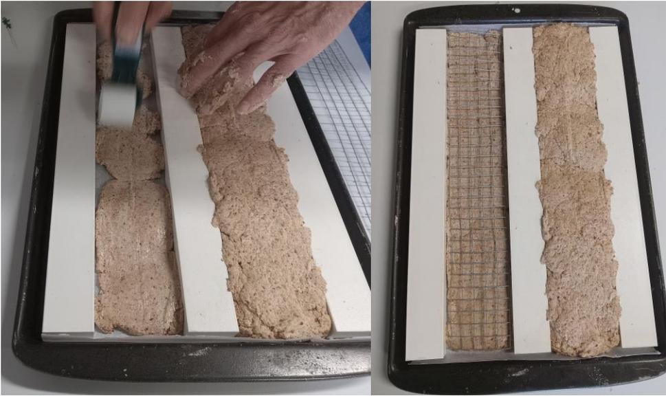
Figure 11. Place reinforcement on thin layer of concrete
