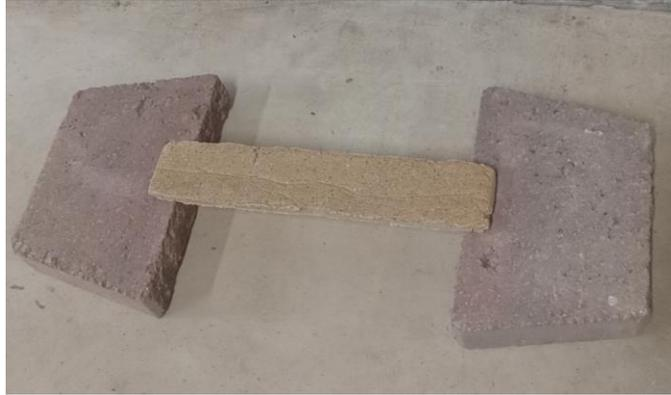
Figure 14. Set the unreinforced specimen across a 13" gap
