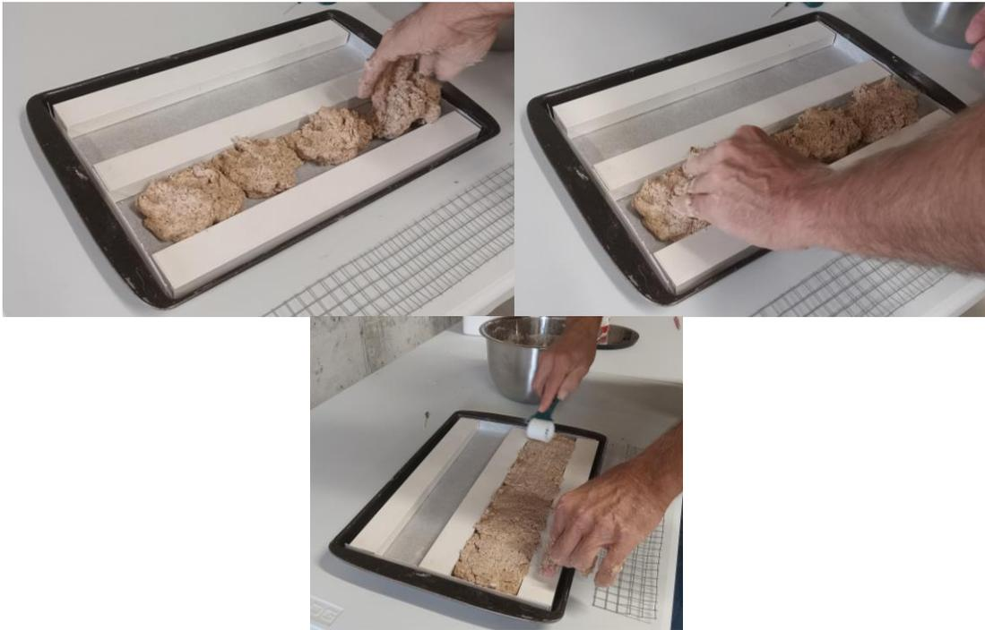
Figure 10. Place, press and roll concrete for unreinforced specimen
