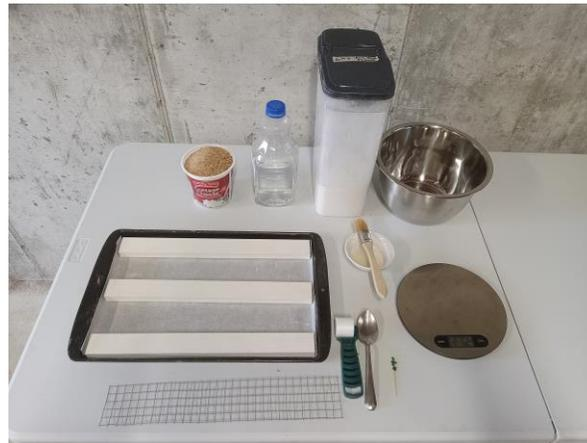
Figure 1. Materials for Flour Concrete Activity
