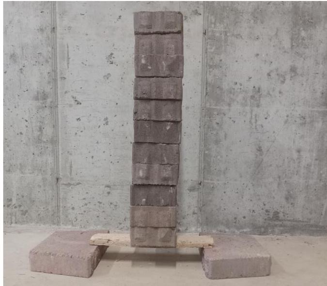
Figure 16. Reinforced beam loaded with 77 pounds
