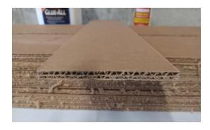
Figure 2. Cut 4" wide strips aligned with the corrugations, as shown
