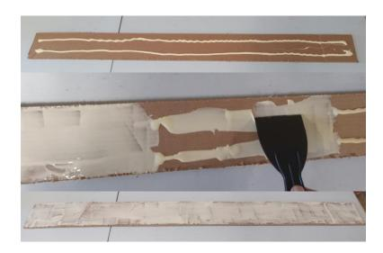
Figure 3. Apply a thin layer of glue over the entire surface
