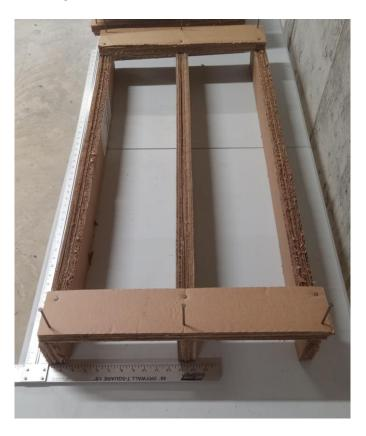
Figure 9. Align the joists and deck boards
