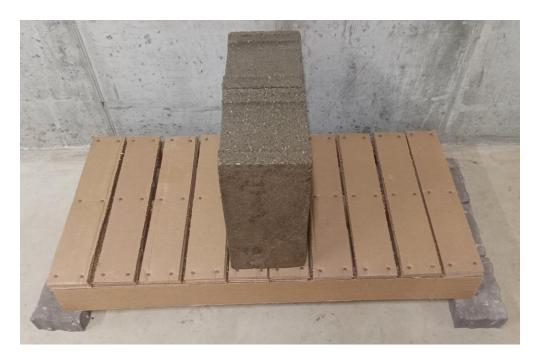
Figure 12. Proof test the bridge with 2 standard concrete blocks
