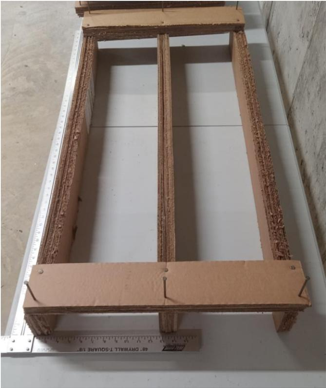
Figure 9. Align the joists and deck boards
