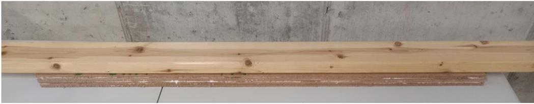
Figure 4. Weight the completed piece and allow to dry
