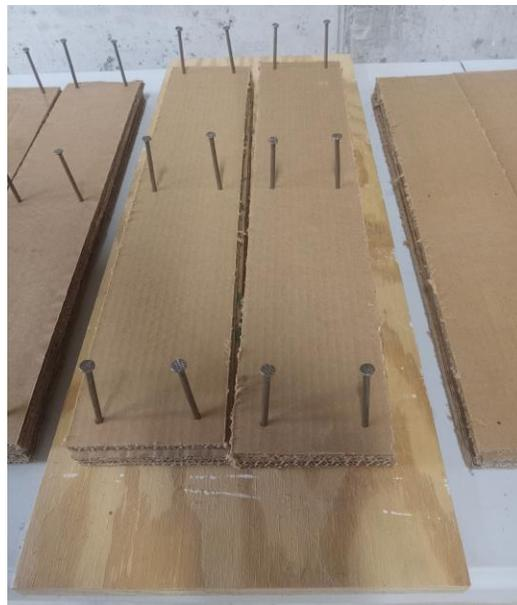
Figure 7. Start nails in deck boards
