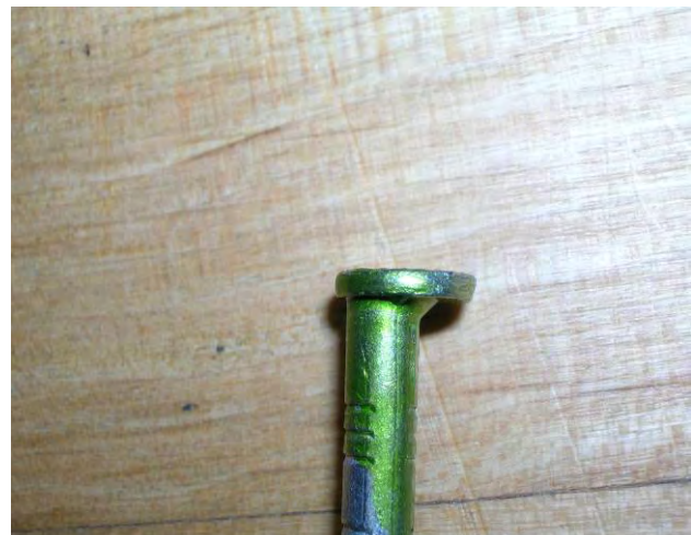
Figure 7 – Asymmetrical full round head of Paslode 16d ring-shank nails
