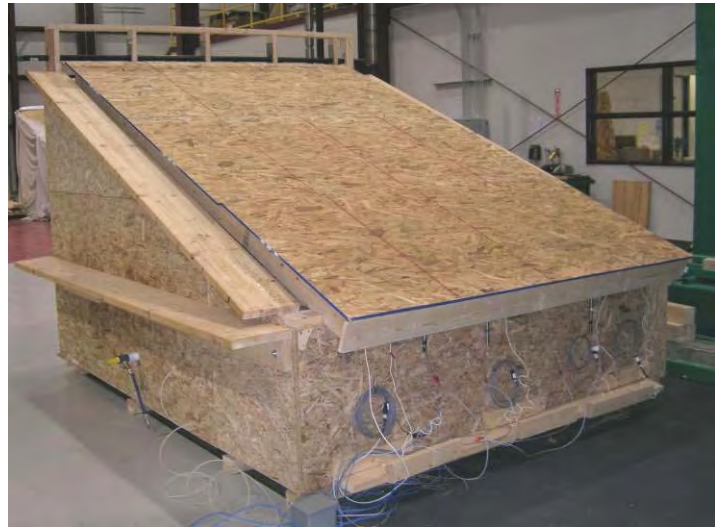
Figure 5 – Uplift specimen ready for testing
