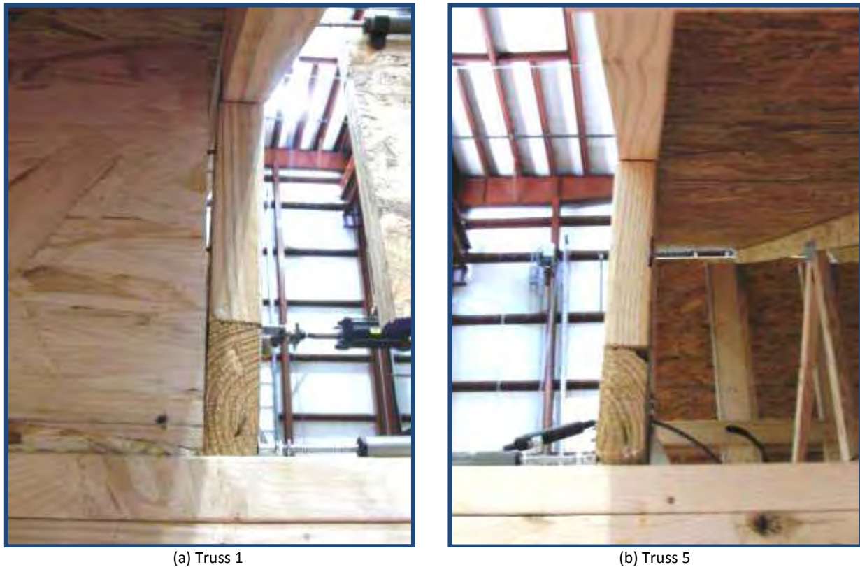
Figure 19 – Comparison of truss heel rotation (Specimen F)
