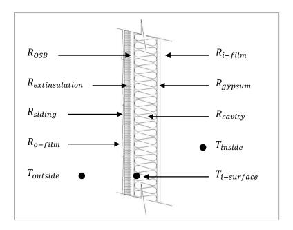
**Figure 47. Condensing Surface Calculation Parameters**
