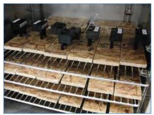
Figure 9. Sensors in the Environmental Chamber for Calibration
