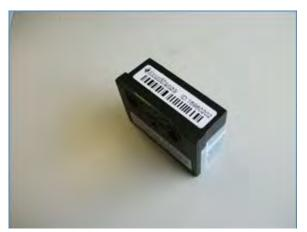
Figure 7. Omnisense S-900-1 Sensor
