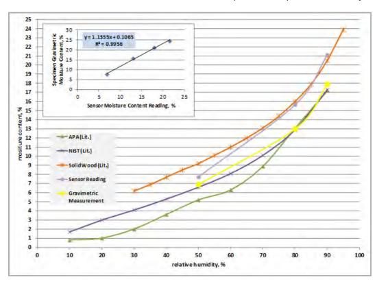
Figure 10. OSB Moisture Content Sensor Calibration Curves
