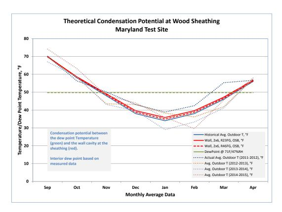
Figure 50. MD Test Site, Theoretical Condensation Potential
