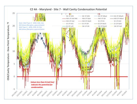
Figure 51. MD Test Site 7, Measured Condensation Potential
