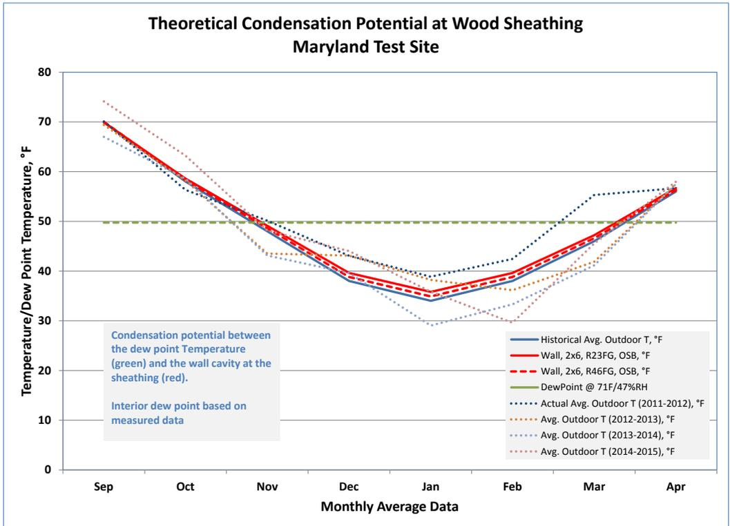
Figure 50. MD Test Site, Theoretical Condensation Potential
