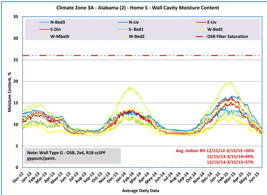
Figure 37. Daily OSB Moisture Content for Climate Zone 3A, AL (2), Test Home 5
