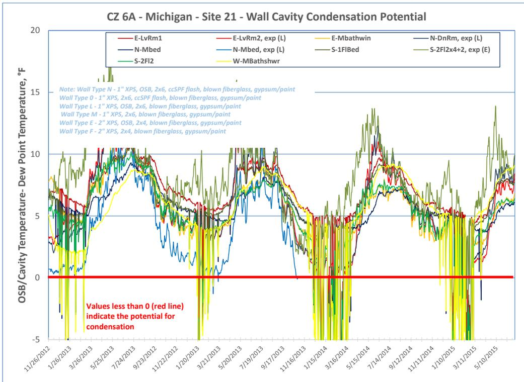
Figure 49. MI Test Site 21, Measured Condensation Potential
