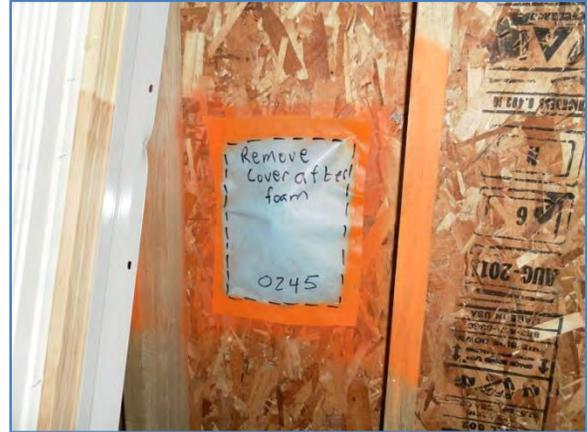
**Figure 4. Sensor Installed in OSB Sheathing That Will Not be Foamed Over in This Cavity**
