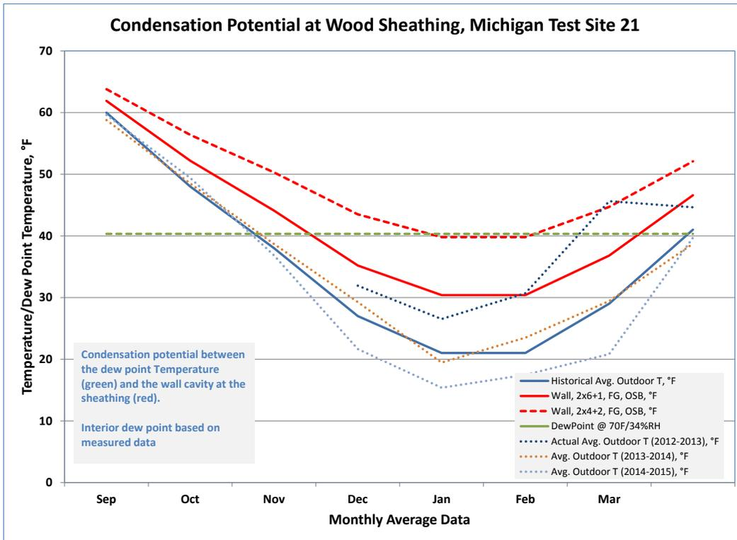
Figure 48. MI Test Site 21, Theoretical Condensation Potential
