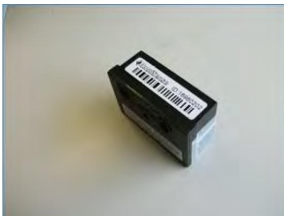
Figure 7. Omnisense S-900-1 Sensor
