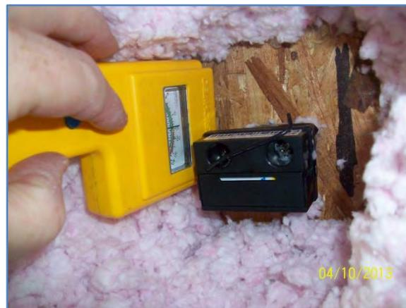
**Figure 55. Moisture Meter Reading Correlated with Sensor**
