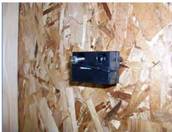
Figure 8. Screws used to Install Moisture Sensors
