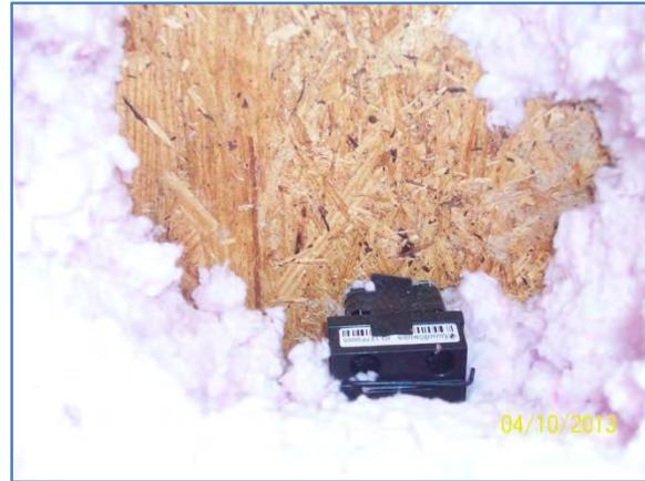
**Figure 54. Moisture Sensor Located**
