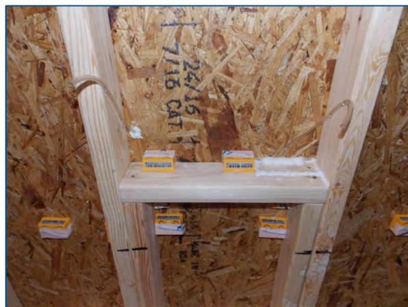
**Figure 10. Water Injection Tubes in Test Walls**
