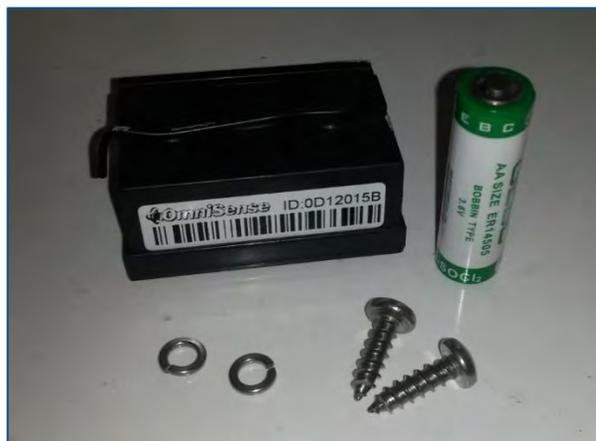
**Figure 6. Wireless Temperature, Humidity and Wood Moisture Sensor**
