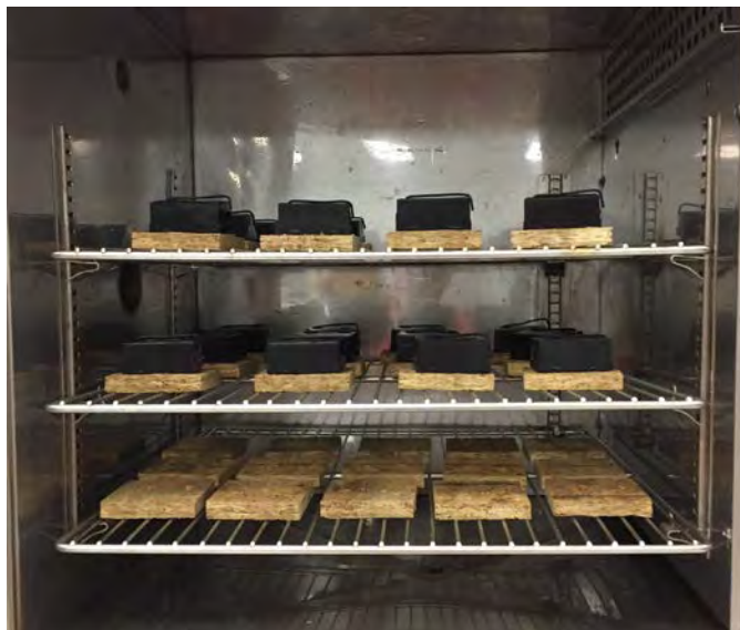
Figure 11. Sensors in the environmental chamber for calibration
