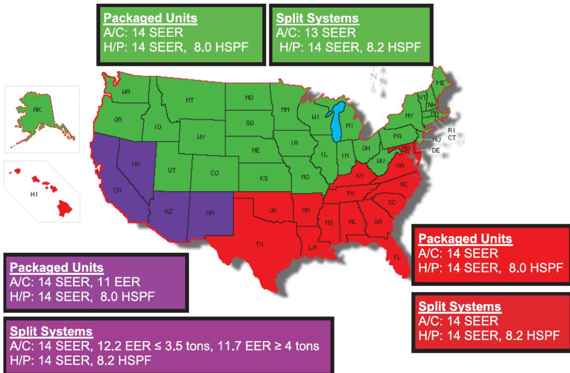
Figure 3. 2015 Federal Minimum Equipment Efficiencies (Illustration: American Standard)
