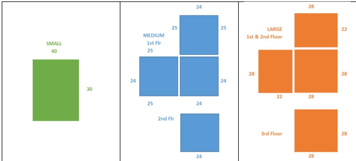
Figure 2. Geometries of the Three Reference Houses
