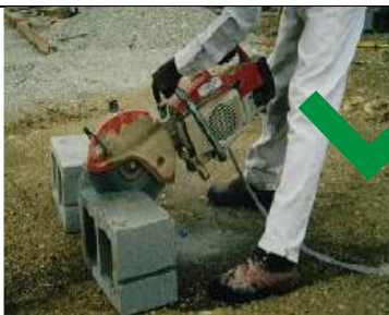
Worker using a handheld masonry saw with water application to blade controls.
