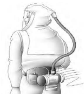
Hood Powered Air-Purifying Respirator (PAPR) APF= 25
