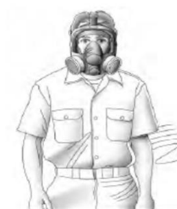
Full facepiece (Elastomeric) APF=50 Needs to be fit tested
