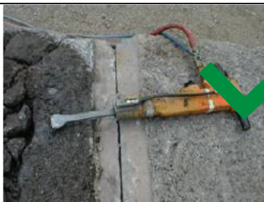
Jackhammer equipped with water spray delivery system.
