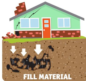
If foundation movement and related structural distress occur, it typically takes many years to develop. Early Development of structural claims is likely indicative of a significant drainage problem, severe over-irrigation or improperly compacted fill material.
