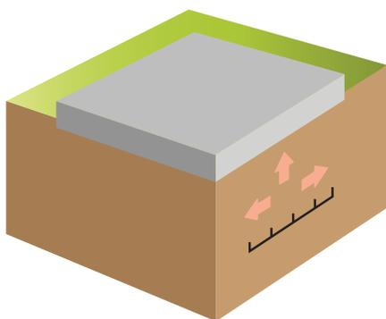
**Most foundations are designed for up to 1" of soil movement. In highly expansive soil areas, slab foundations can be designed for up to 4 inches of soil movement**
