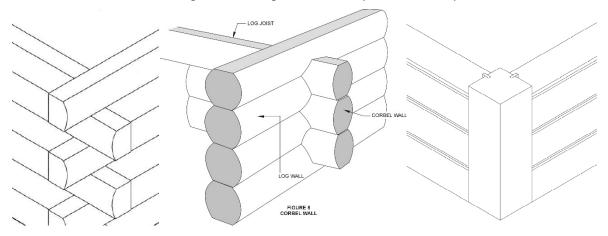
Fig. 4.5.1.1 Example of a Butt & Pass (left), an Interlocking (center, graphic by Randy Kaatz), and a Posted (right) corner.
