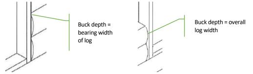
Figure 4-7 The depth of the rough buck relative to the log profile will affect the method of sealing and trim.
