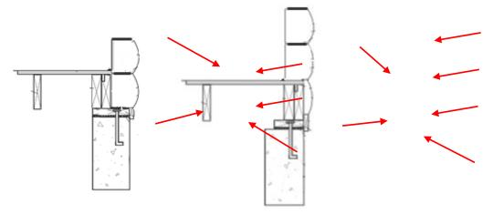
Fig. 4.2.1.1 Examples of sill log (left) and bottom plate log (right). The arrows point to potential sources of air and water leaks. Log suppliers and builders have various methods and materials they use to seal these locations. Ask them for their details/construction manual.
