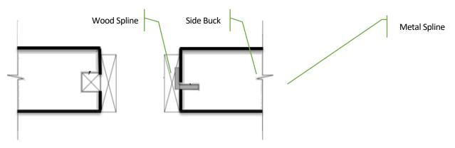
Figure 4-8 Options for connecting the log ends to the buck that offer alignment and vertical movement.
