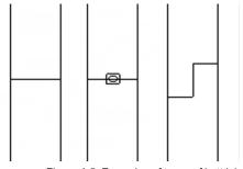
Figure 4-5 Examples of types of butt joints: square trim, spline, and scarf.
