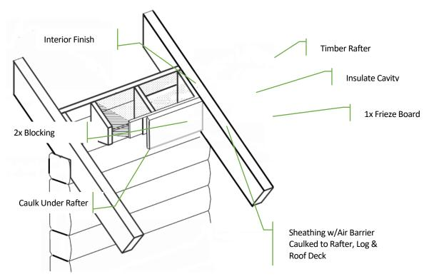
Figure 4-2 Rafters to Log Wall: An air seal is required at the bottom side of decking and between log/timber rafters when used.
