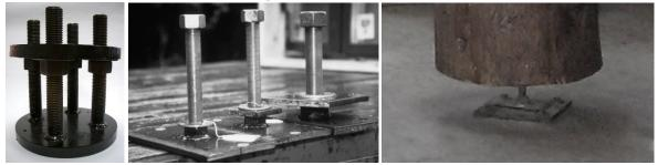
Fig. 4.3.2 Types of settling jacks.
