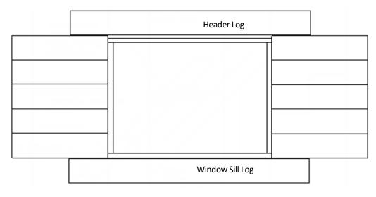
Fig. 4.3.3.3. Header logs and window sill logs need to extend past the wall opening. The header log requires sufficient length to accommodate bearing of the load on the log below. Both logs must extend to allow proper installation of fasteners.
