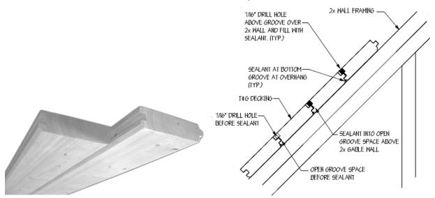
Figure 4-3 The seal between the gable end wall and T&G decking is critical. Some systems use a gasket while others use a drill and caulk method. The detail illustrates a framed gable, but the same technique is applicable to any wall construction where T&G decking passes over it.
