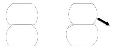
Fig. 4.1.3.1. Example of stacking logs to create overhangs or ledges. Slope ledges on outside to promote drainage.
