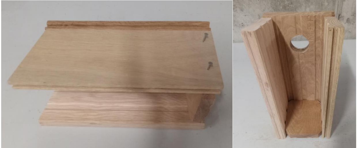
Figure 7. Nail the bottom to the sides
