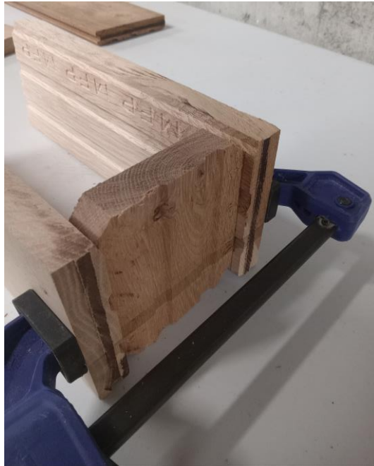
Figure 5. Clamp the sides to the floor
